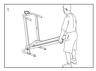
Hold the treadmill securely with your left hand as shown. Insert the Storage Pin (42) into the hole in the right side of the Right Upright (36) and into the Frame (29) as far as it will go.
